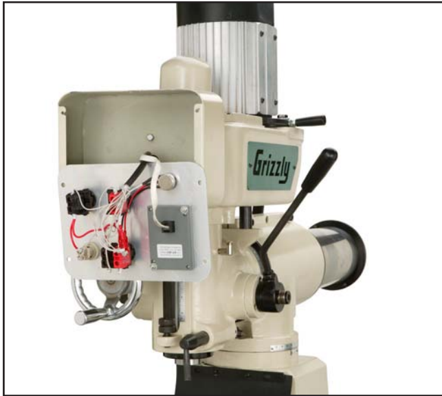
Figure 68. Control panel wiring.
